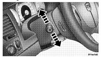
Move the lever up or down to signal a right-hand or left-hand turn.
